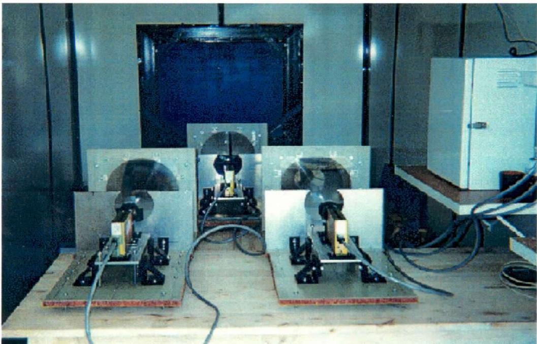
**The APF light source includes three separate light sources at ~330nm, 360nm and 390nm.**
