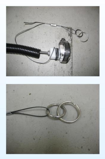
• Diffuser is secured by the hose clamp.
